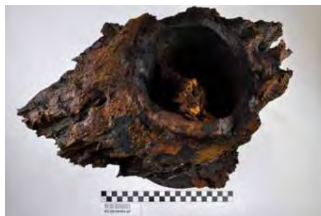
Fig. 104. Wood and graphitized iron hatch roller base BC-05-00169-ML (Diam. 19.2 x 18.9cm).
