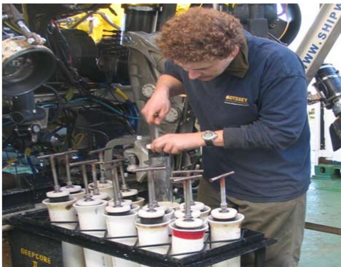
Fig. 15. Preparing environmental core tubes for descent onto the wreck.
