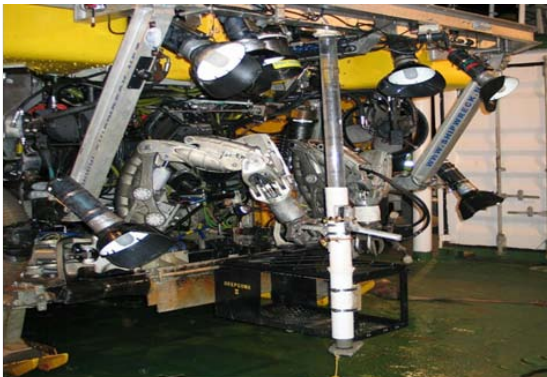
Fig. 16. A 2m 'long core' installed on ROV Zeus for descent onto the wreck site.
