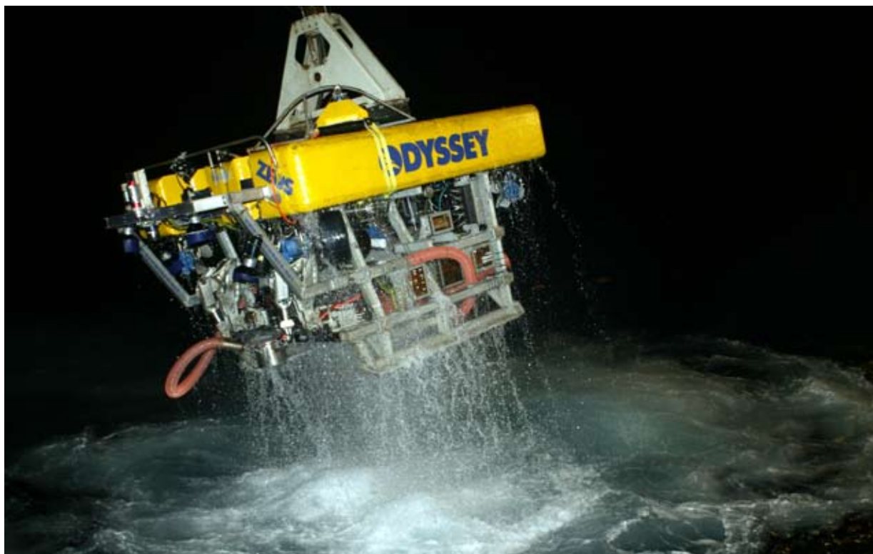
Fig. 5. The 7.26-ton, 3.7m-long ROV Zeus used during the survey and excavation of the Republic.
