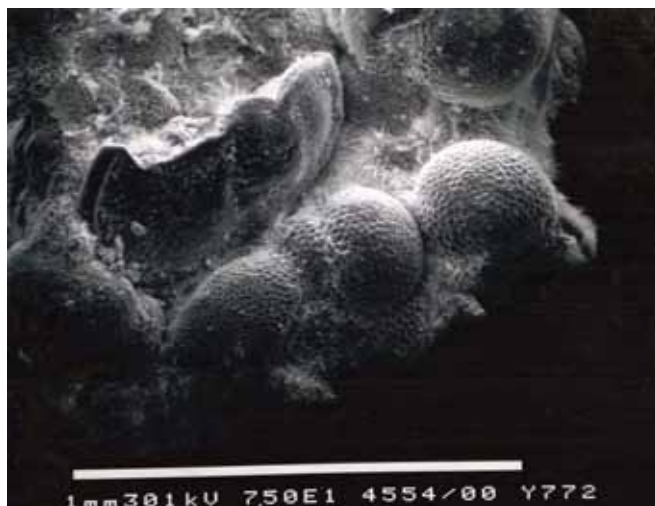
Fig. 8. Skeletons of marine coral on the outer surface of a silver coin encrustation examined by SEM (x 75).
