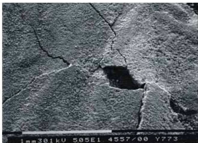
Figs. 10-11. Iron oxide and iron sulfide deposits identified on a silver coin encrustation examined by SEM (x 50).
