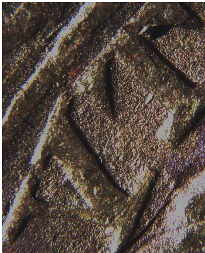
Fig. 6. Mirror image of the letters 'TY' from the word 'LIBERTY' preserved on the inside encrustation of a gold coin examined under an optical microscope.
