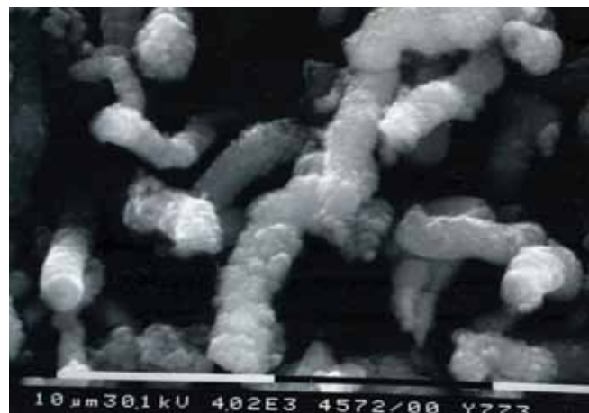
Fig. 24. Tubular iron oxide particles deposited on a silver coin examined by SEM (x 4,000).
