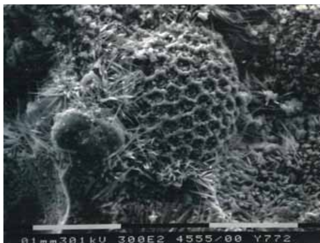
Fig. 9. Skeletons of marine coral on the outer surface of a silver coin encrustation, fractured open to reveal the walls of coral cell chambers inside. Examined by SEM (x 300).
