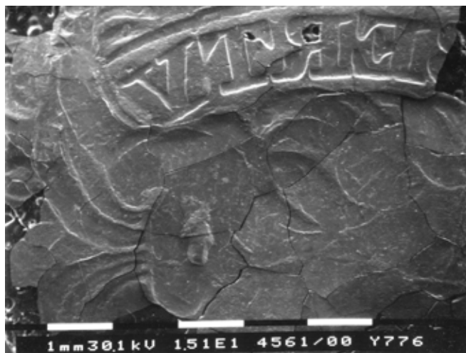
Fig. 20. Inner surface of a gold coin concretion with engraving marks preserved in mirror relief, examined by secondary electron detector (x 15).
