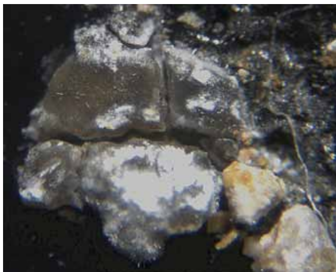
Fig. 2. Upper side of encrustation, crystalline in nature, from a silver coin examined under an optical microscope.
