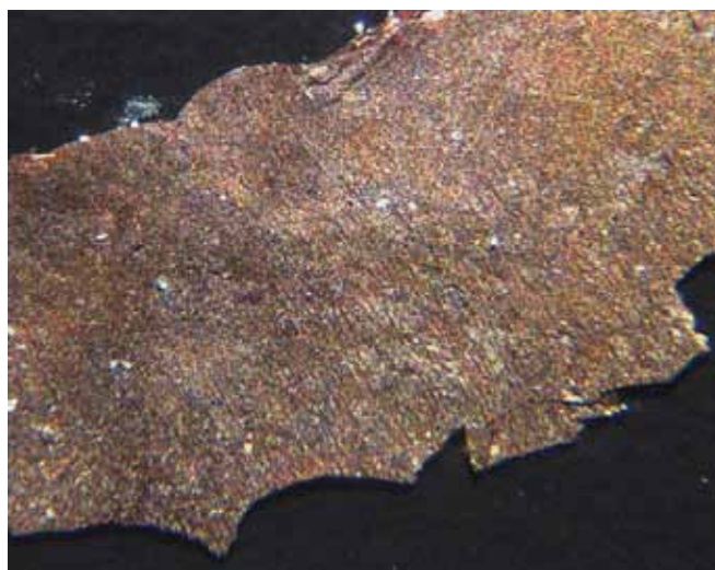
Fig. 1. Upper side of encrustation from a SS Republic shipwreck gold coin examined under an optical microscope.
