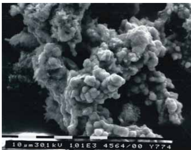
Fig. 13. Deposits with sulfur- and iron-rich particles probably formed by bacteria on a silver coin encrustation examined by SEM (x 1,000).
