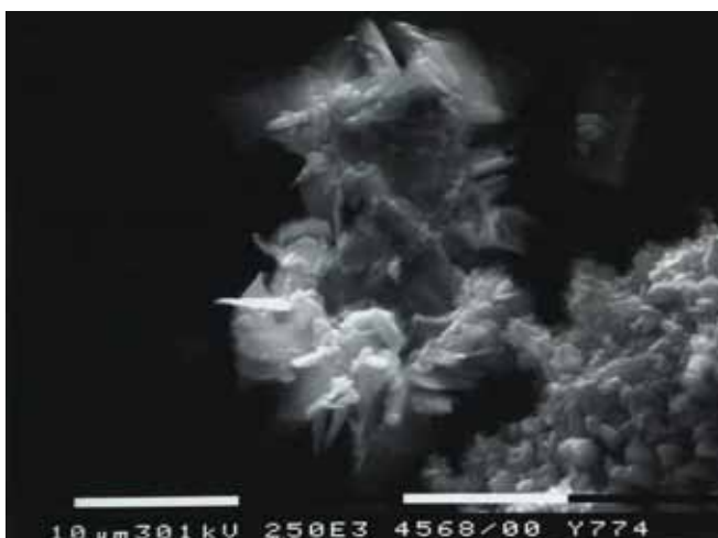
Fig. 15. A small deposit of silver sulfide crystals identified on a silver coin concretion examined by SEM (x 2,500).
