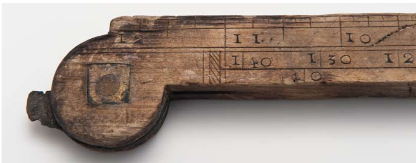
Fig. 6. Detail of the hinge mechanism at the folding end of side A.
