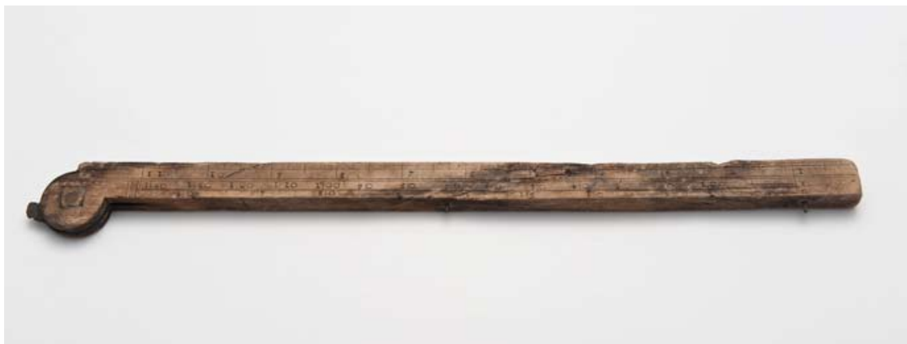
Fig. 1. Site 35F wooden folding rule side A with an incised inch scale numbered [0]-12 inches and divided into half, quarter and eighth units.
