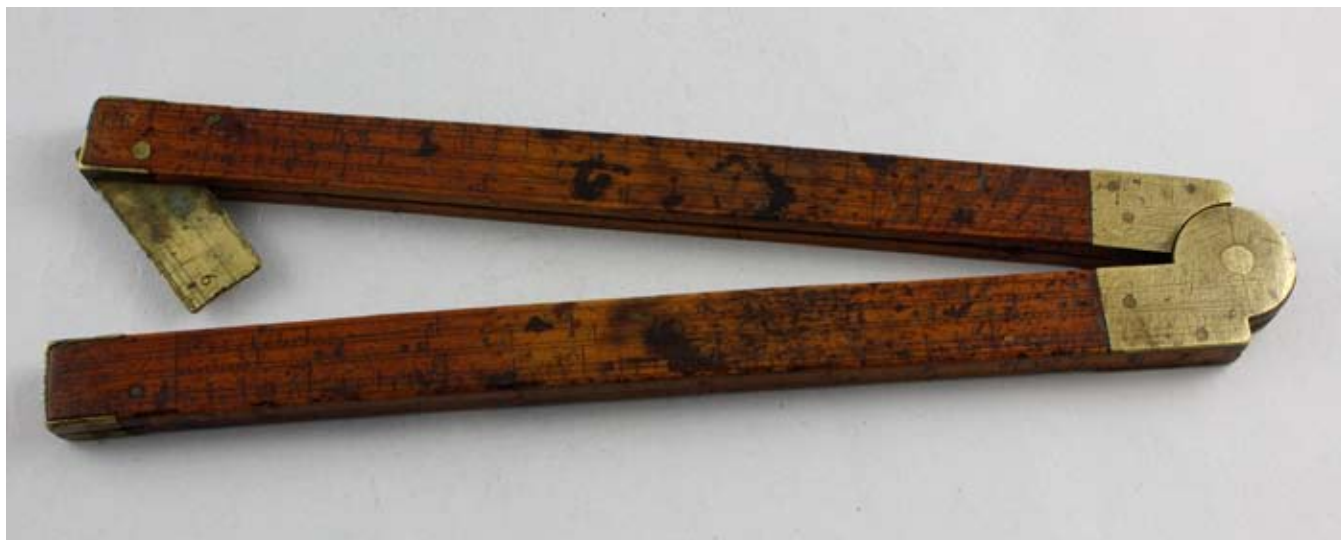
Fig. 18. A three-fold rule at Colonial Williamsburg (inv. 1997-100) with inch scale to 18in and the remains of a 6in brass extension piece. The central 'circle-square' scales are unlabelled. Photograph: permission of the Colonial Williamsburg Foundation.
