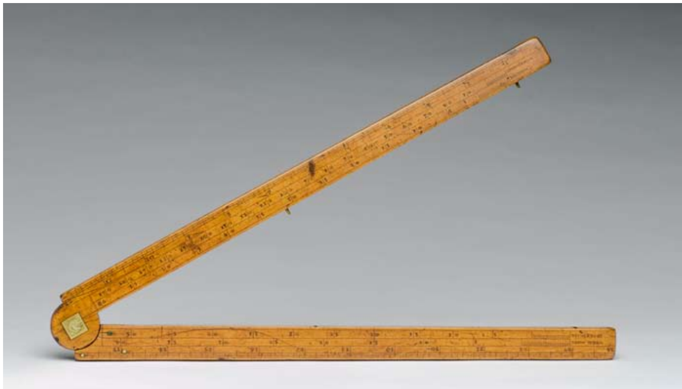
Fig. 16. An intact wooden folding rule in the collections of the Science Museum, London, was crafted to the same design as the site 35F instrument, and is dated by an inscription to 1659. Its four central scales are fully labelled as circumference, diameter, square equal and square within. Photo: © Science Museum, London (inv. 1954-292).
