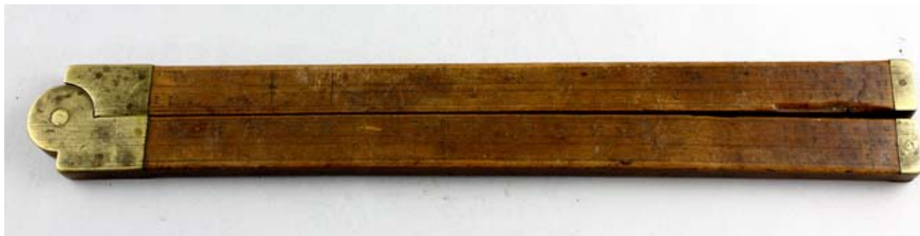
Fig. 20. A two-fold, 2ft rule engraved 'N P 1678' in the collection of Colonial Williamsburg (inv. 1995-18). This carries the same arrangement of scales as the site 35F rule, here showing the face with timber and board lines and tables. Photograph: permission of the Colonial Williamsburg Foundation.
