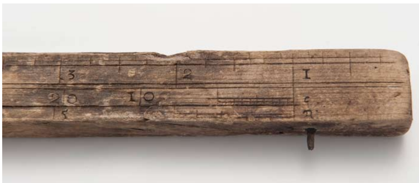
Fig. 10. Detail of the end section of side A with a pair of scales incised 'C' and 'D', standing for 'Circumference' and 'Diameter'.
