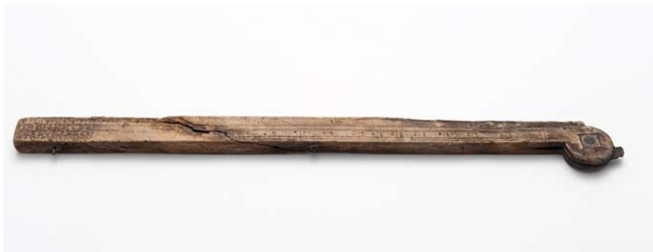
Fig. 2. Site 35F wooden folding rule side B incorporates three elements. Inner scale: the end of a line of board measure running from 12 to 36, each unit subdivided to half. Outer scale: beginning of a line of timber measure from 9 to 12, each unit subdivided to quarter. Far left: table of timber undermeasure.
