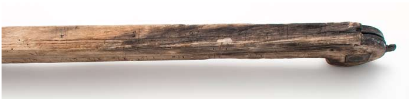
Fig. 4. Detail of the side edge of the folding rule incised with a logarithmic line of numbers 1-10. (The missing leg would have carried the same scale to make a double radius line 1-100.)
