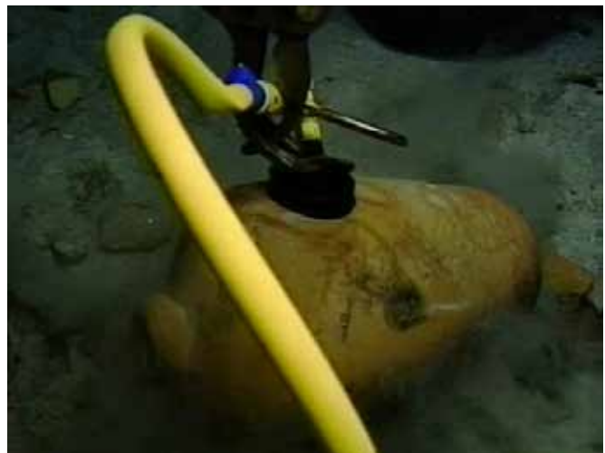
Figs. 20-21. An evolved small limpet suction bellows device used to recover artifacts from the Tortugas shipwreck inspired from paper printing industry technology.
