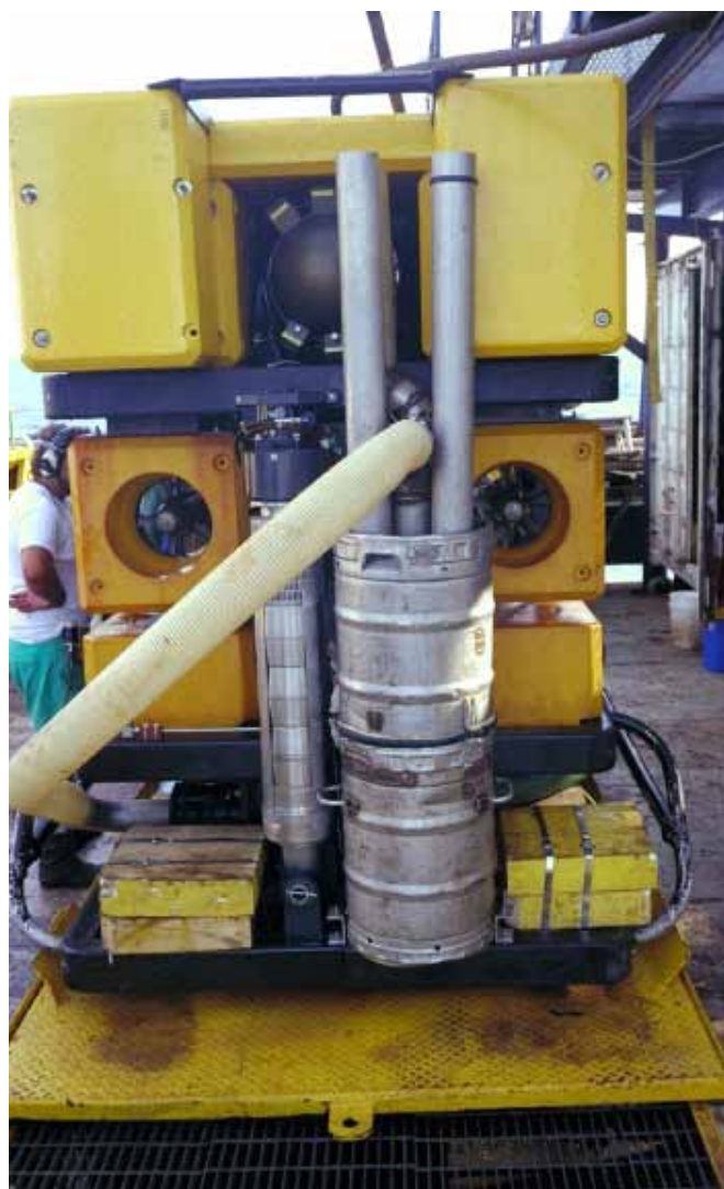
Figs. 10-11. The custom-designed receiver and venturi pump from the SeRF (Sediment Removal and Filtration System) unit installed onto the rear of the ROV Merlin (with an early prototype at top). Photo (Fig. 11): John Astley.
