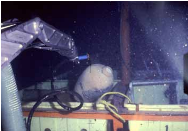
Fig. 24. An olive jar being secured into a 4Plex unit by the ROV Merlin using its limpet suction device.
