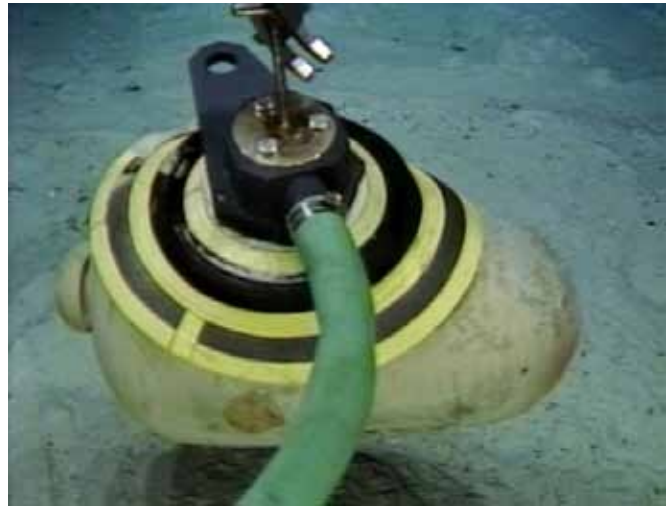
Fig. 19. An early limpet suction device developed for the Tortugas project being used to recover an olive jar.
