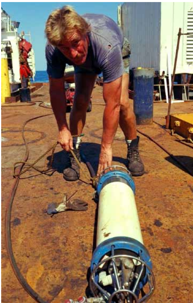
Fig. 16. Alan Crampton rigging a Sonardyne transponder for deployment. Photo: John Astley.
