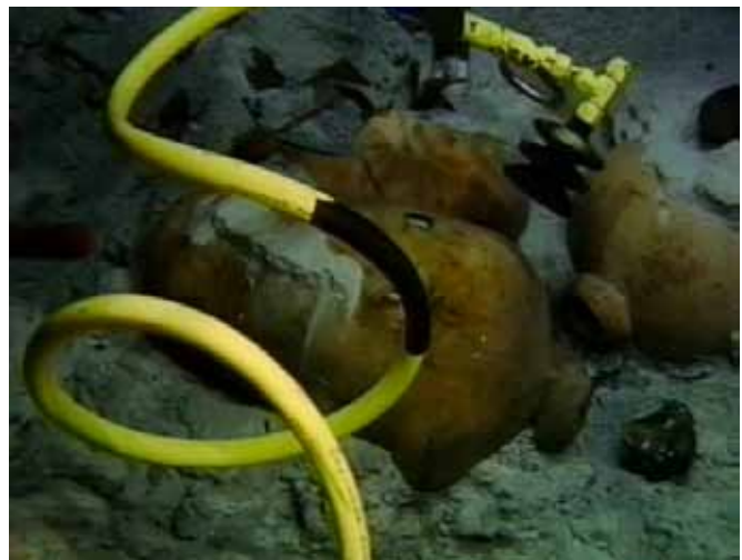
Fig. 19. An early limpet suction device developed for the Tortugas project being used to recover an olive jar.
