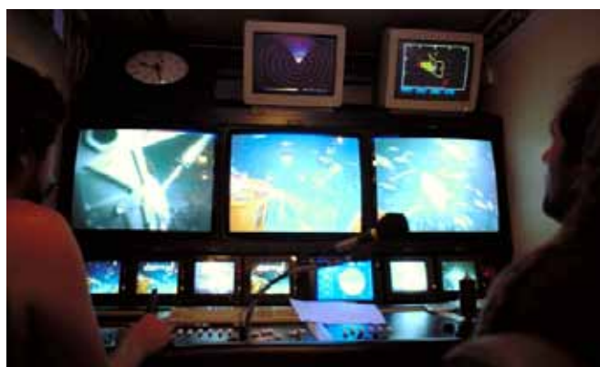
Fig. 14. Monitoring archaeological operations on the Tortugas shipwreck from the Seahawk Retriever. The top screens displayed sonar and navigation. The three middle colour screens revealed a very wide view of the site under investigation. The lower row of screens depicted compass, vehicle instrumentation and stern camera data, plus other cameras monitoring the ROV parts. In the foreground the datalogger runs four SVHS recorders and the logging system. Photo: John Astley.
