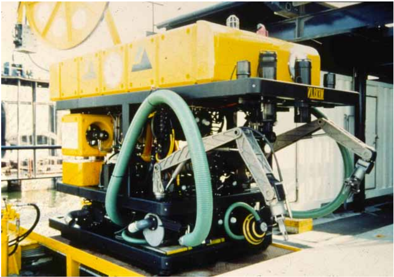
Fig. 7. The 3-ton ROV Merlin built for the Tortugas shipwreck excavation; with its SeRF system hose and nozzle at front right, two manipulator arms and limpet suction device at center. Along the badge bar are two 35mm cameras and two 70mm still cameras.
