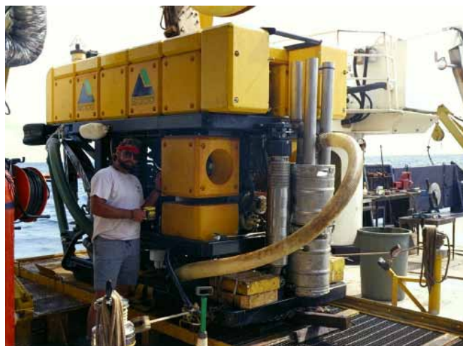
Fig. 9. The SeRF (Sediment Removal and Filtration System) tool for sieving small finds custom-designed for the Tortugas shipwreck excavation and installed onto the rear of the ROV Merlin. Photo: John Astley.
