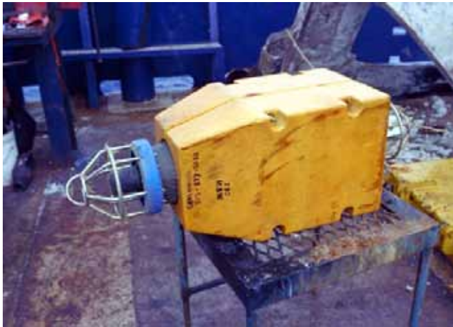
Fig. 15. A Sonardyne transponder, with the transducer at left and the hook release at right, all encased in a buoyancy jacket to facilitate recovery. Photo: John Astley.
