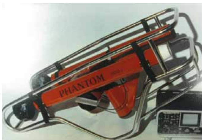
Fig. 4. A DOE Phantom 300 ROV used for visual reconnaissance from the RV Seahawk.
