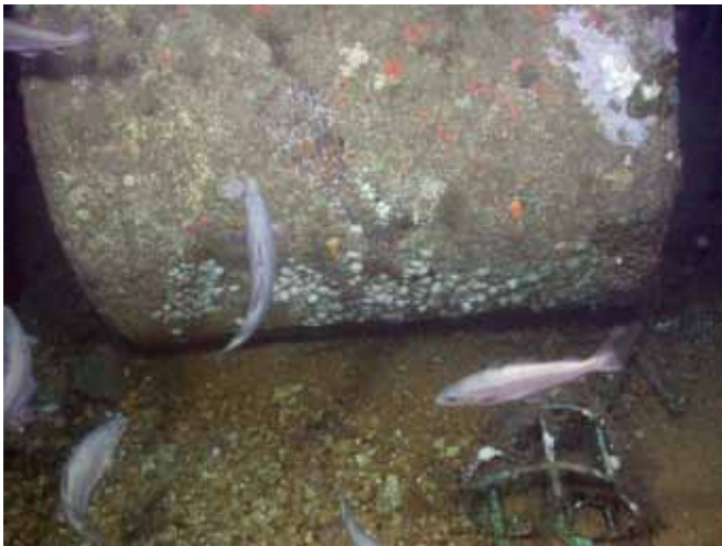
Figs. 14-15. Scotch boiler outside the starboard center of the wreck, with a lobster creel snagged to one side.
