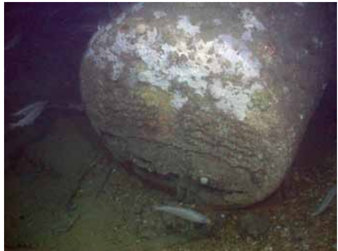
Figs. 14-15. Scotch boiler outside the starboard center of the wreck, with a lobster creel snagged to one side.
