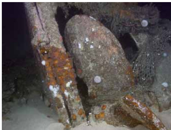
Fig. 18. Detail of the rudder turned hard to port and the ship's four-bladed propeller.
