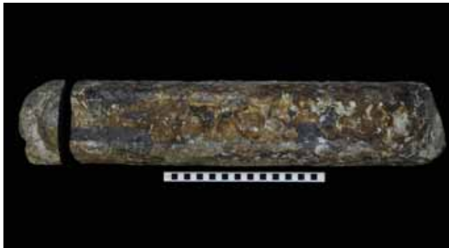
Fig. 26. Lead ingot DAN-05-0001-ML, L. 75cm. The metal has been sampled for alpha emissivity testing.
