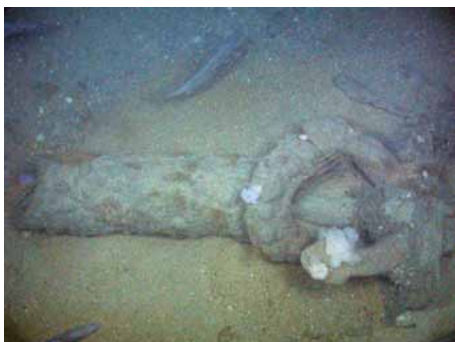
Fig. 22. A stockless anchor stowed inside a collapsed hawse pipe in the port bow section of the wreck (2008: top), and newly snagged with fishing net in 2015 (bottom). Sections of steel hull panels behind.
