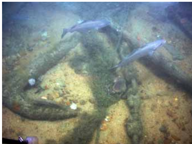
Fig. 10. Kedge anchor off the portside bow attached to chain, on which fishing net is snagged.
