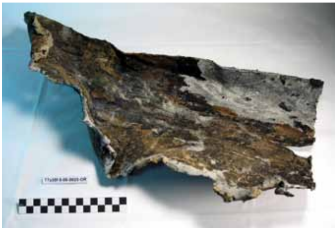
Figs. 24-25. Lead hull repair patches recovered from the site (Th. 0.8cm).
