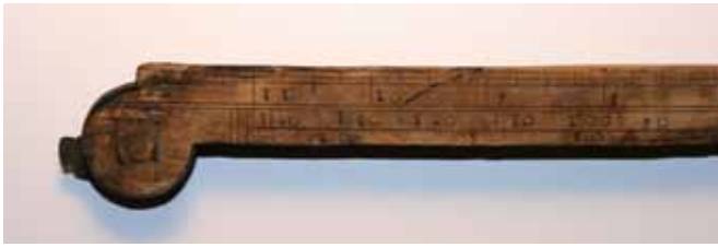
Fig. 53. Detail of the hinge and inch scale on side A of the folding wooden rule.
