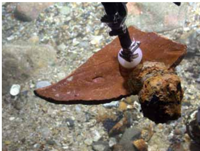
Fig. 12. ROV Zeus' limpet suction system recovering a typically preserved potsherd.
