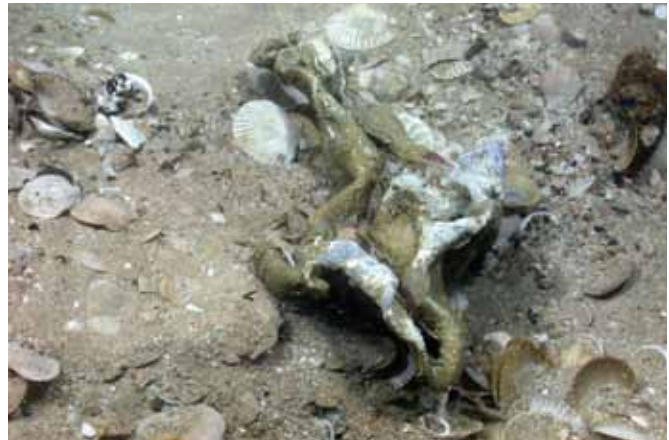
Fig. 23. A lead hull tingle patch in situ.
