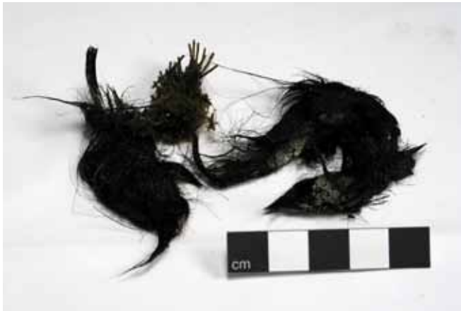
Fig. 22. Animal hair (possibly horse) used as caulking between wooden planks.
